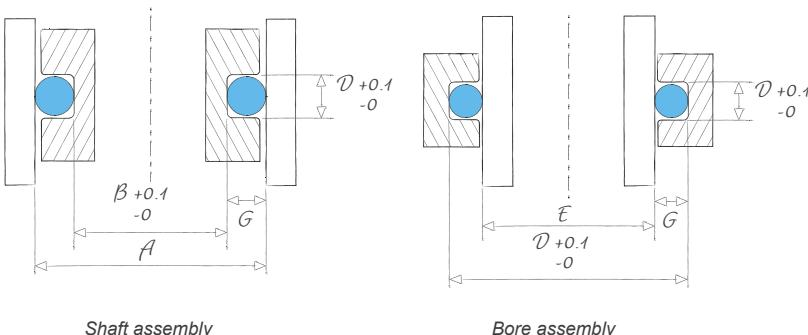
While the dimensions shown will suit most applications, the combined effects of temperature, pressure and the fluid mean that validation by testing is required (O-Ring compound and dimensions).
