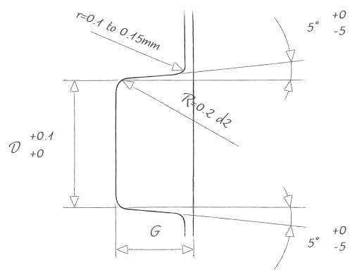
Groove dimensions for radial (shaft / bore) assembly in dynamic applications.
