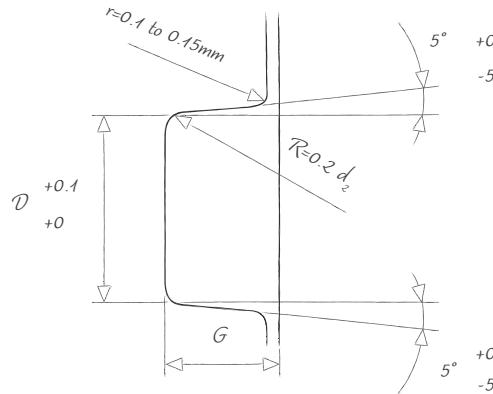
Groove dimensions for radial (shaft / bore) assembly in static applications
