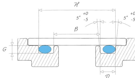
Groove dimensions for axial assembly (cover)
