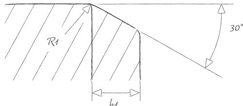
Chamfer on shaft
