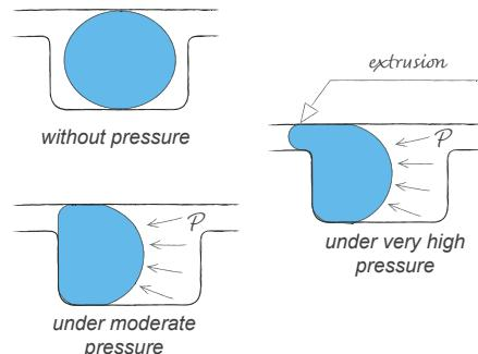
*The higher the pressure, the more the clearance needs to be reduced, the more the hardness needs to be increased.*
